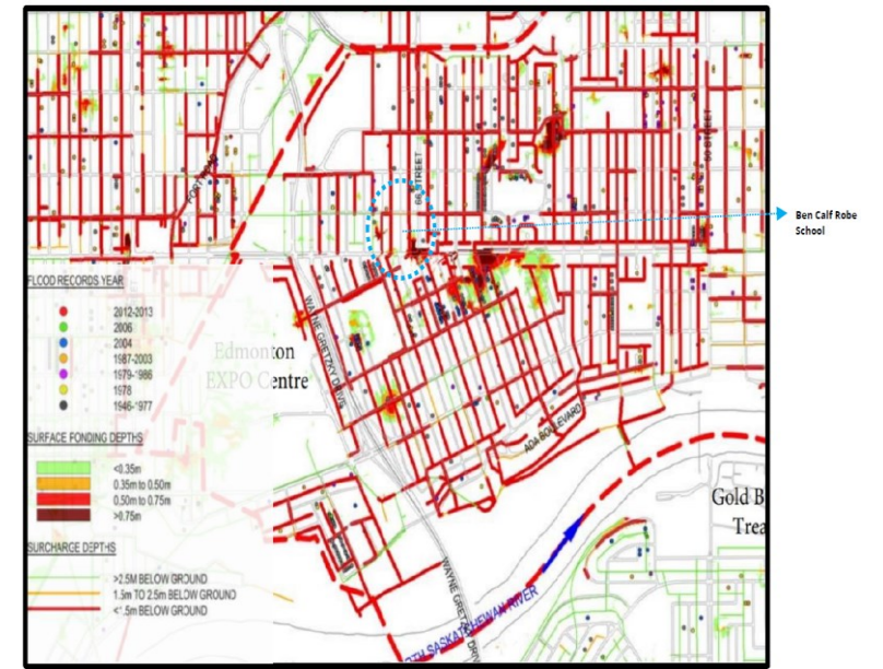
Figure 9: Flood records, surface ponding and sanitary surcharge (EPCOR for City of Edmonton, n/d)
